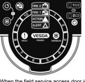
When the field service access door is open, the user has access to the RESET (), DISABLE 🖲, Fire Test 📾 , AutoLearn 🚫 and Instant Fault Finder functions When the Instant Fault Finder function is activated, the Smoke Dial converts to a fault indicator, with the dial segment numbers corresponding to the faults listed below.
